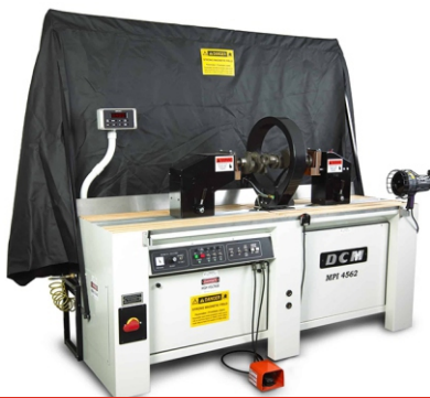
Crack Detection (MPI)
